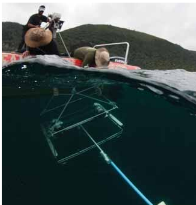
Rig split: A Baited Remote Underwater Stereo Video system (stereo-BRUVs) is retrieved after being left on the seabed to film for an hour. These systems sample fish abundance, size and species composition and are the primary sampling method used in SAEON's long-term monitoring programme in the Tsitsikamma National Park Marine Protected Area. Photo: Steve Benjamin.
