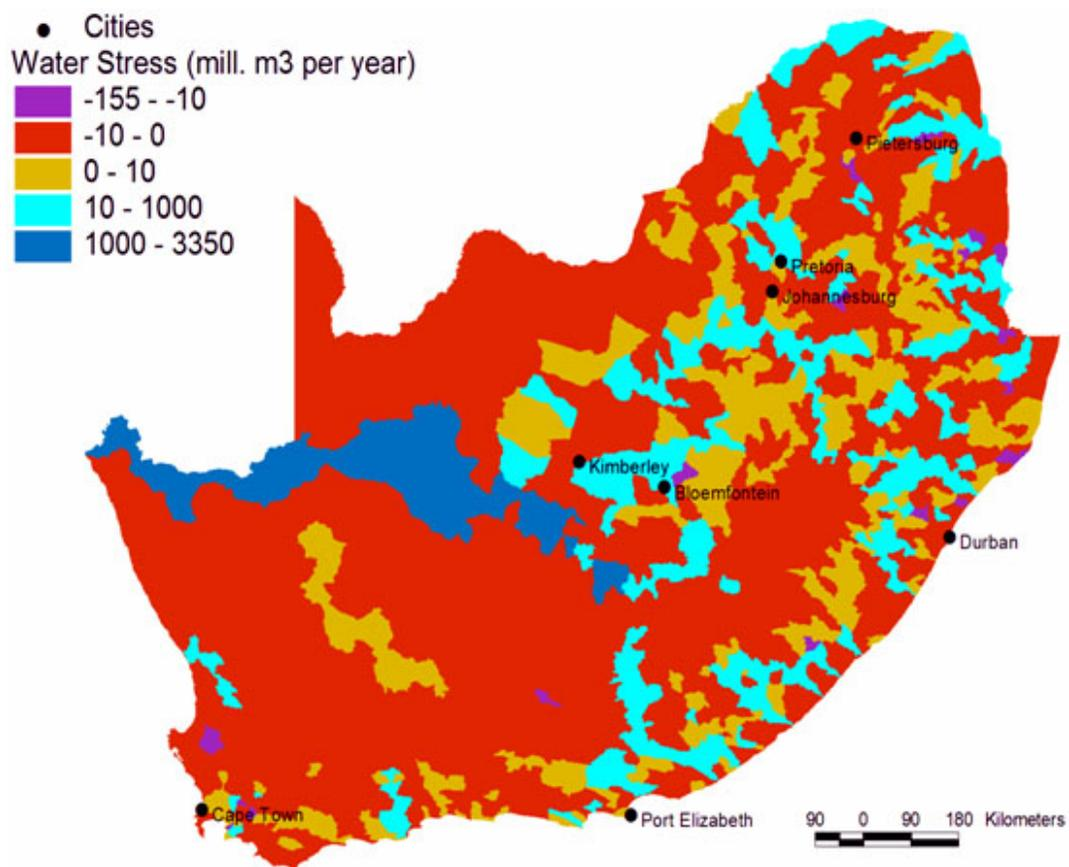
Figure 1.2: The 2005 annual water balance in South African Catchments, where water stress occurs when the demand for water exceeds the amount that is available, and is measured in this figure by million cubic meters per year, with purple and red showing high amounts of water stress (Council for Scientific and Industrial Research (CSIR), 2014).
