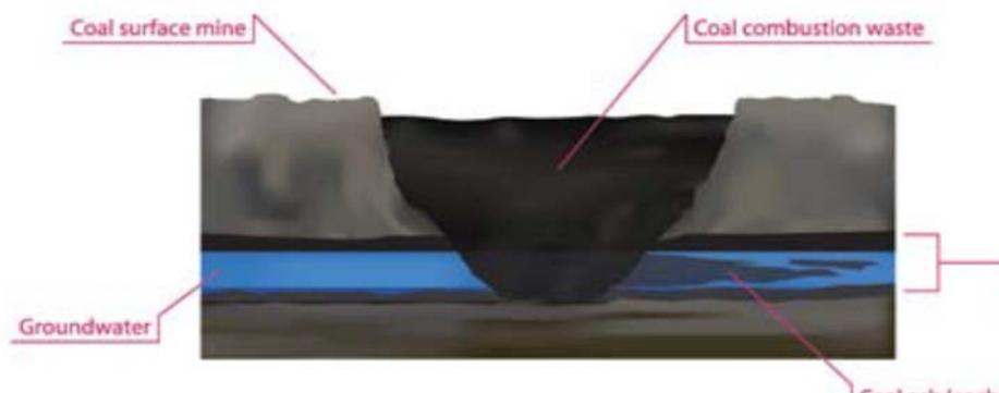
Pit backfilling and its potential to pollute groundwater (Earth Justice, 2009).
