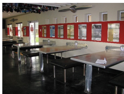
Fig. 15. Interior view with Tables Constructed from Aircraft Panels Supported by Alloy Propeller Blades
