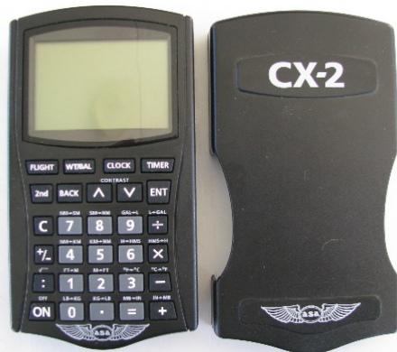
Fig. 24. CX2 Pathfinder Flight Computer
