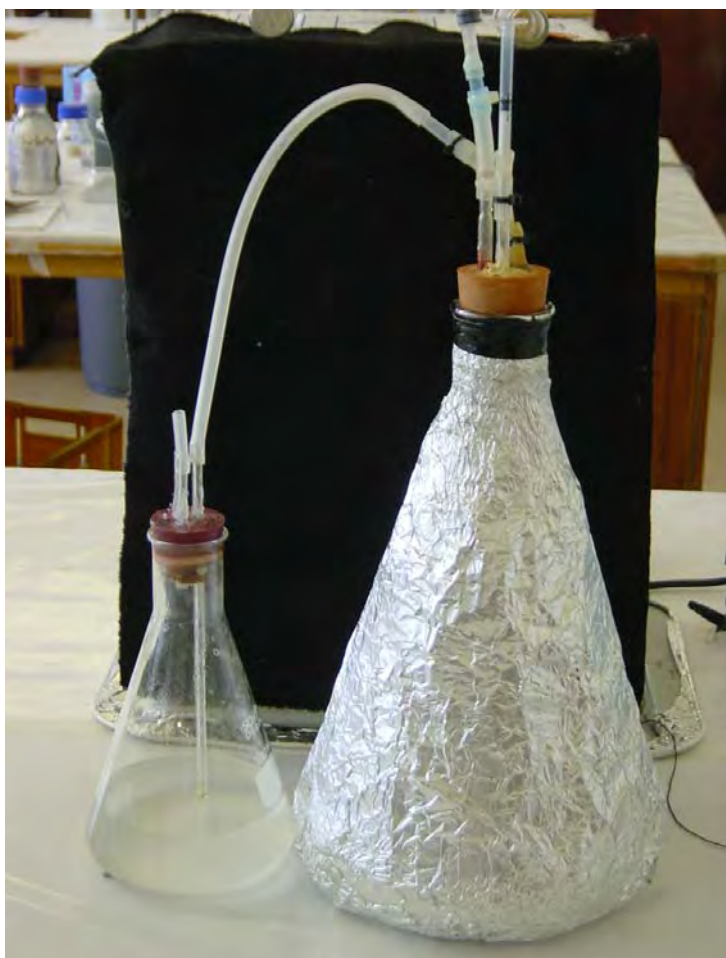
Figure 2.1 5L-batch reactor used as cell generator showing syringes for sampling and nitrogen flushing, with an adjoining smaller flask containing zinc acetate to trap sulphide.
