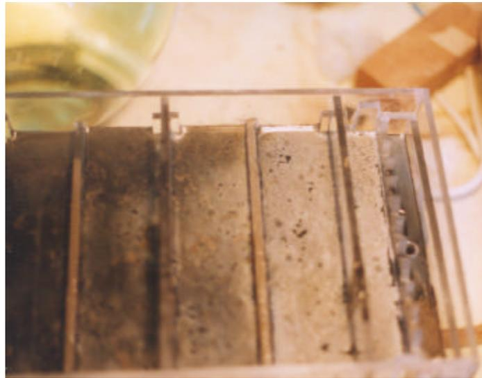
**Figure 2.5:** Biofilm formation on the surface of the Baffle Reactor within 3 hours of start up.
