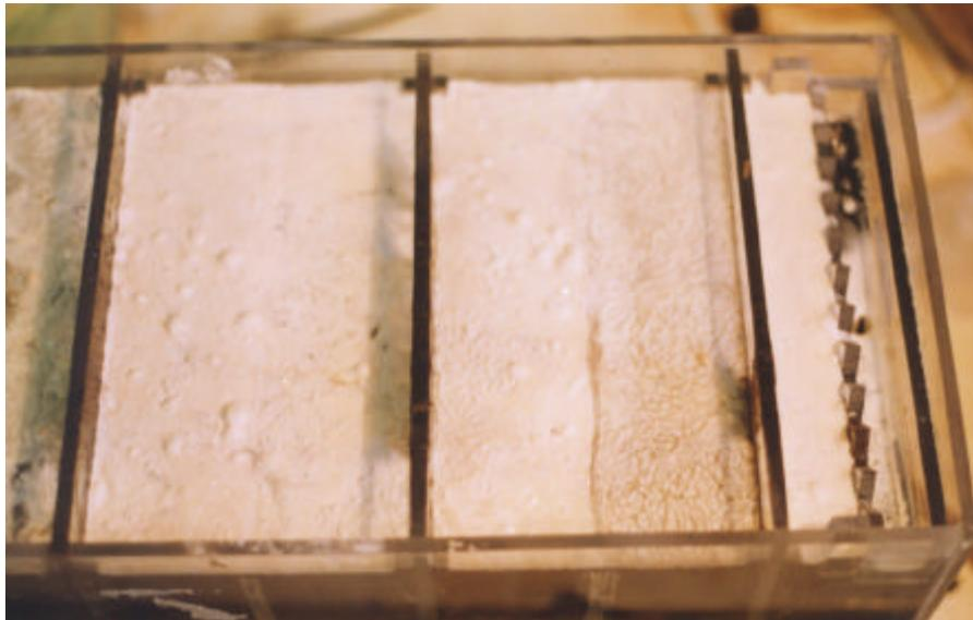
**Figure 2.7:** A Photograph of the floating sulphur biofilm on the surface of the Baffle Reactor 2 days after start up.
