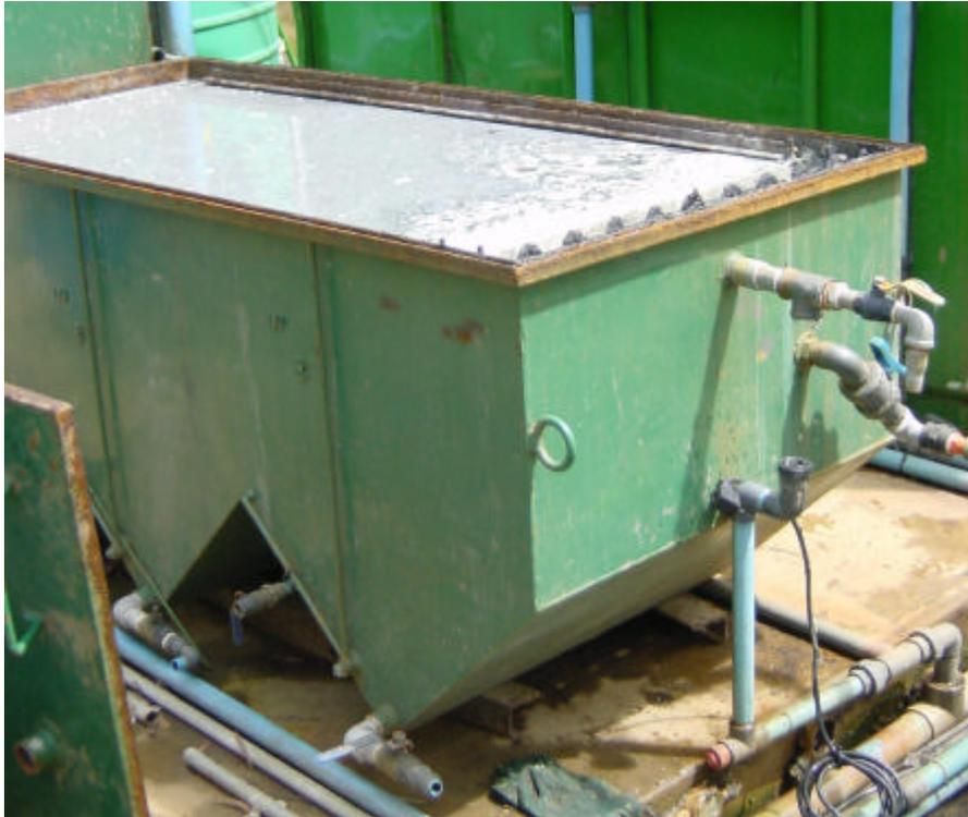
**Figure 2.13:** The Scaled-up version of the Baffle Reactor.
