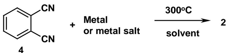
**Scheme 1.5:** Preparation of MPC from phthalonitrile (**4**).
