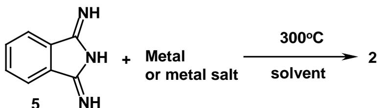
**Scheme 1.6:** Preparation of MPC from 1,3-diiminoisoindoline (**5**).
