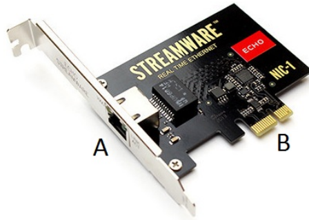
Figure 4.6 : An Echo NIC-1 Network Adaptor [6].
