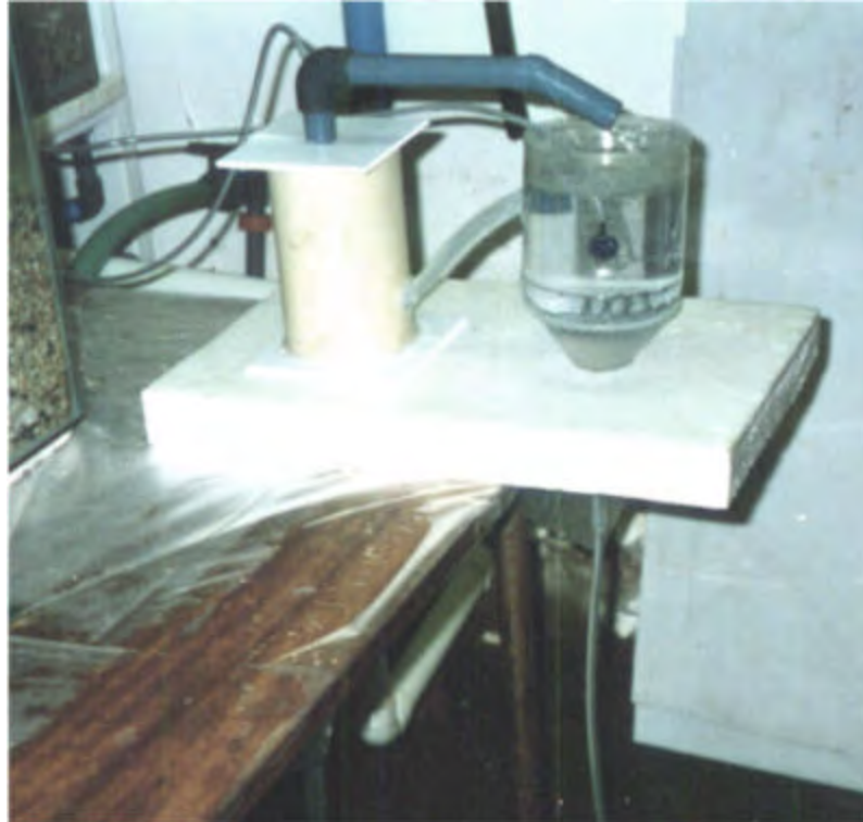
Fig. 1 Illustration of 2-l conical plastic tank with biological filter tested in Method 1.
