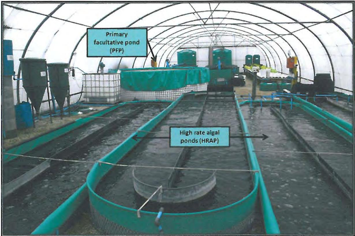
**Figure 1.5.a:** Project Eden: Anaerobically digested effluent was fed into a primary facultative pond (PFP) and high rate algal ponds (HRAP).
