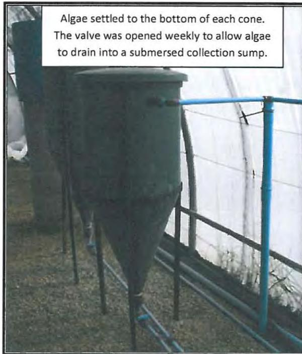
**Figure 3.1.m:** The algal settling cones used to harvest algae from the high rate algal ponds.
