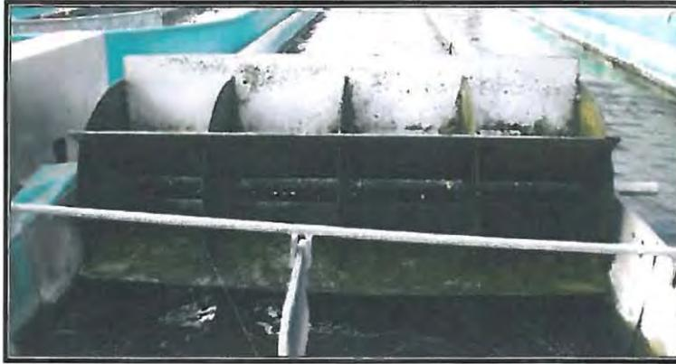
**Figure 3.1.j:** An example of one of the paddle wheels used to keep algae in suspension.
