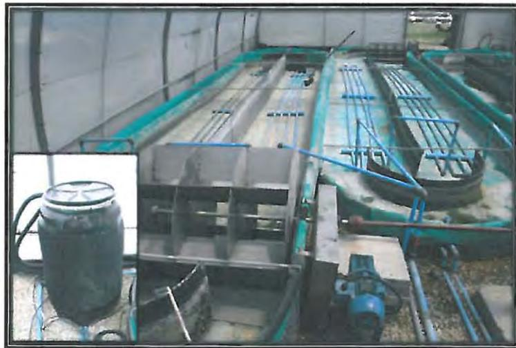
**Figure 3.1.k:** The heating system that was installed in high rate algal pond train-A. The insulated drum geyser that stored heated water from the heat pump (insert).
