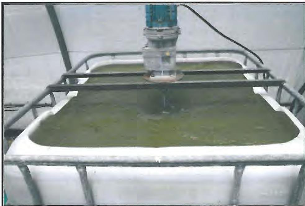
**Figure 3.2.a:** The algal culture with added post-anaerobically digested effluent before inoculation into the high rate algal ponds.
