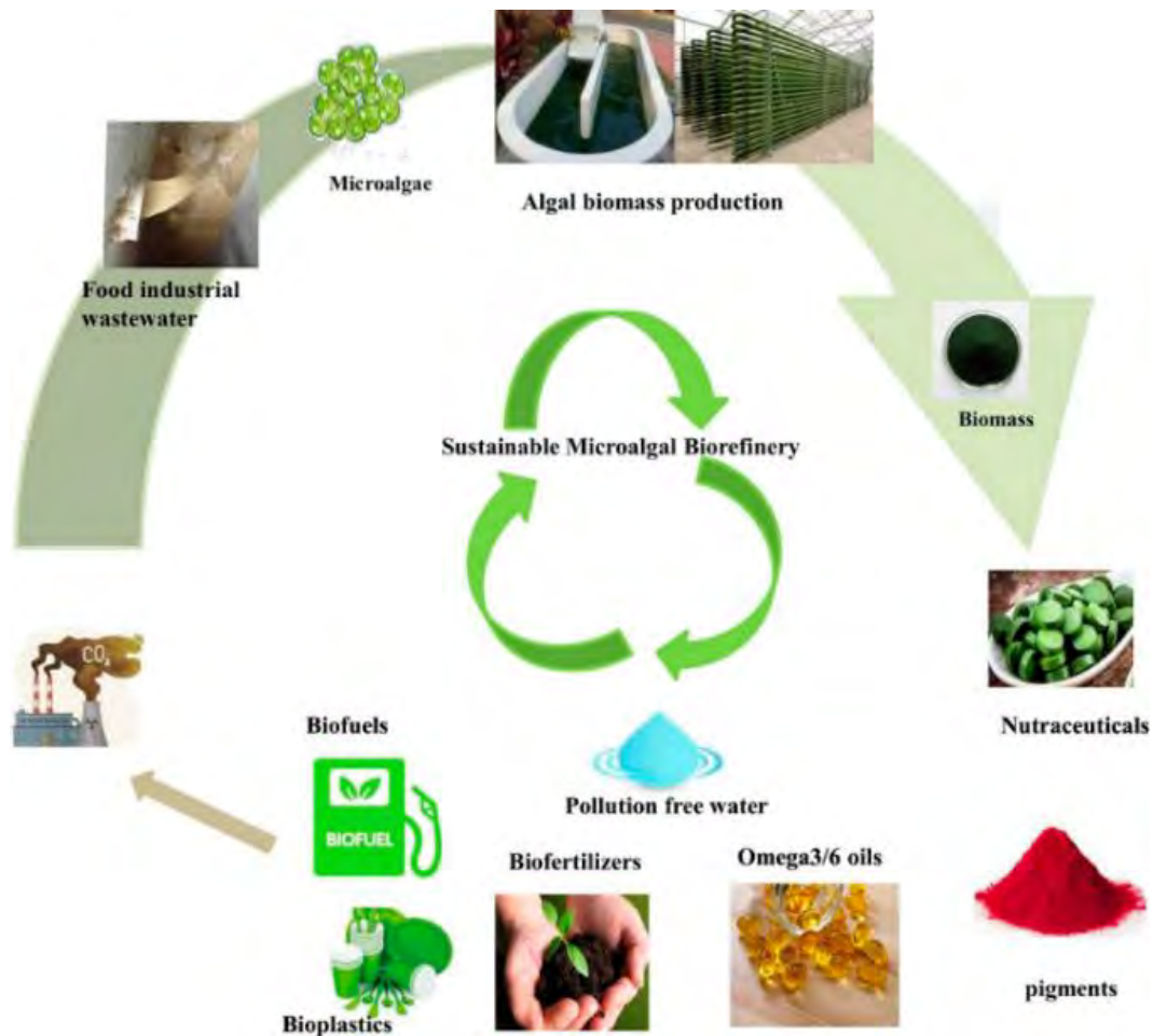
Figure 1.14 Sustainable microalgal biorefinery products coupled with food industrial wastewater [Adapted from Ummalyma et al. (2022)]
