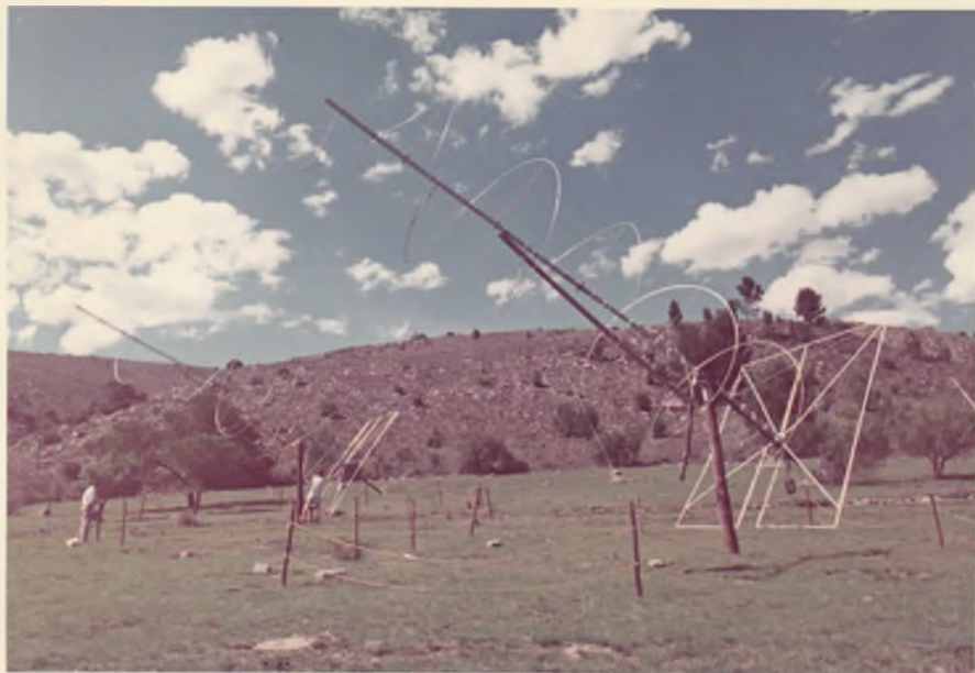
Plate 3. The right- and left-handed polarized helical antennas for the 30 to 45 MHz range.
