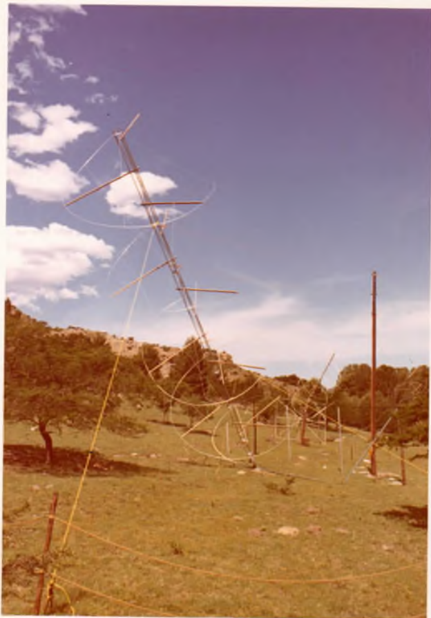
Plate 6. The left-handed helix for the 15 to 26 MHz range.
